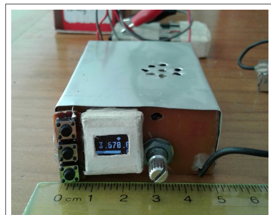
Smallest digital rig. 50X75x26mm. Up/down buttons to tune. Weight 80am.
